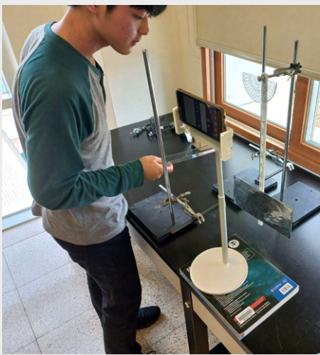
Andy investigated using a magnetic field as a damper for an aluminium pendulum.
